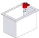
1. Drill the holes for securing it to the edge of the tank as shown in the drawing (see item 4.1.3 and 4.1.4).
