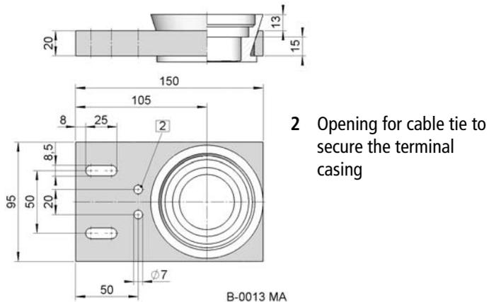
Support SHB/HM for immersion heaters with a nominal immersion tube length of over 800 mm.
