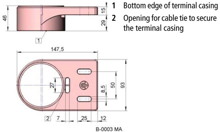
Support HB for immersion heaters with a nominal immersion tube length of up to 800 mm.
